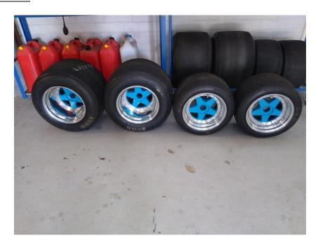
$2 \times 14$ " rear wheels &  $2 \times 10$ " front wheels. Cast centre with new inner and outer rims. Fitted with Avon A11 tyres. \$2,500.
