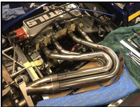
Exhaust fabricating in progress and completed with ceramic coating.
