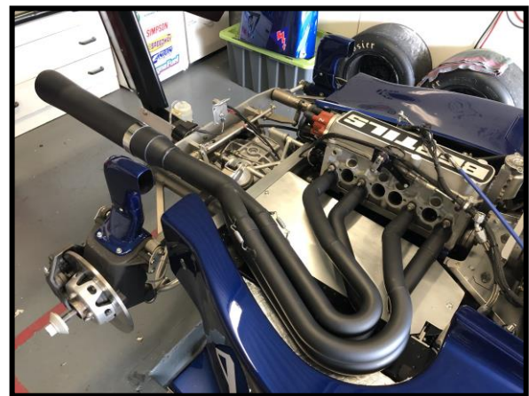
Exhaust fabricating in progress and completed with ceramic coating.
