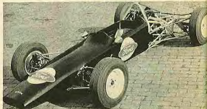
Bill Reynolds' Wren was the first car completed and therefore used by Ford for their publicity blurb. Conventional styling features, very small frontal area, no windscreen. PAUL HARRINGTON
