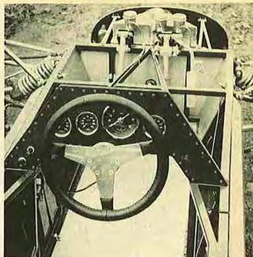
Square tubing, neat and comfortable cockpit design, high standard of overall finish highlight the P4a from Bowin.
